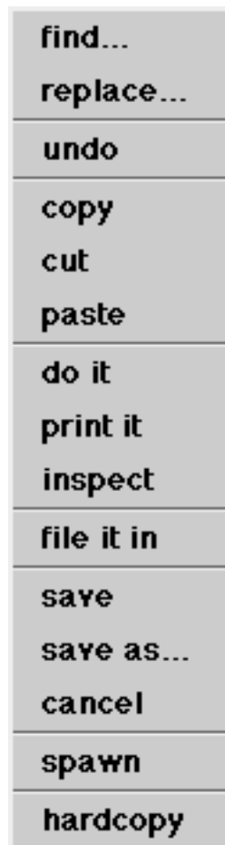
Figure 6.7: The <operate> menu available from the lower pane of the File Browser when a file is selected
